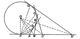
Let O be the centre of the circle. Then, since the angles PA'O, PB'O are respectively complementary to half the angles AOP, BOP, the angle A'OB' is equal to half the angle AOB, and is therefore equal to the angle APB.
